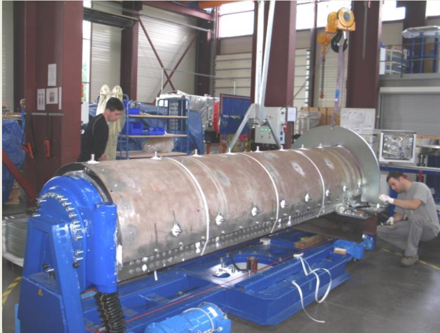
Mold being placed onto Dipole Coil “B” Layers 1&2 in preparation for VPI (May 27, 2014).
