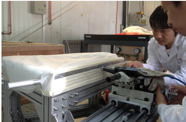
Pining the wire mounts
