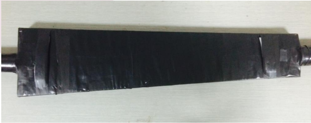
LASPD(Kedi) couple to PMT directly.
