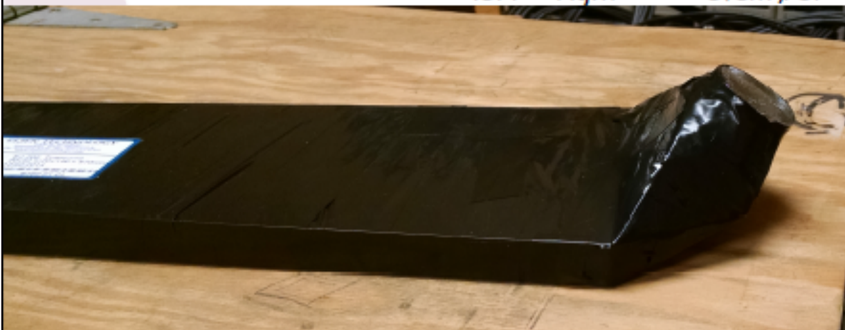
LASPD with 55 degree fishtail light guide
