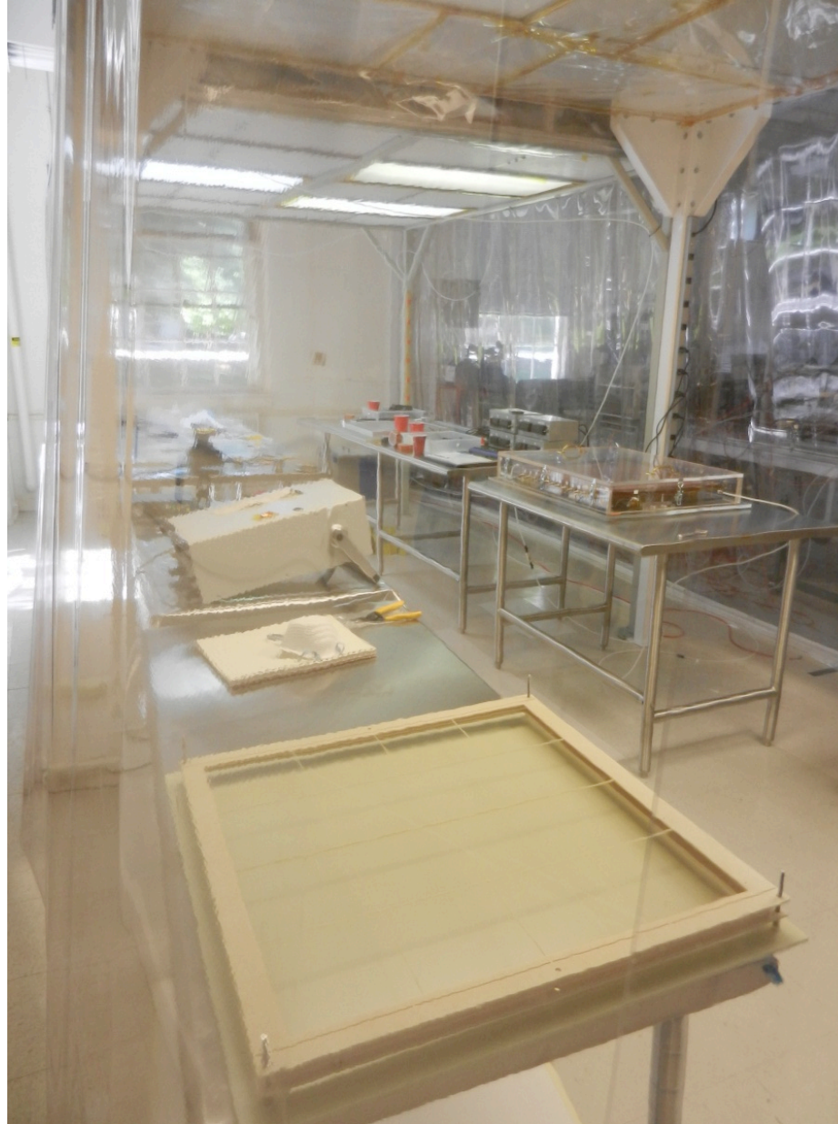
Large area ( 3 \times 7 \text{ m}^2 ) class 1000 Clean Room
