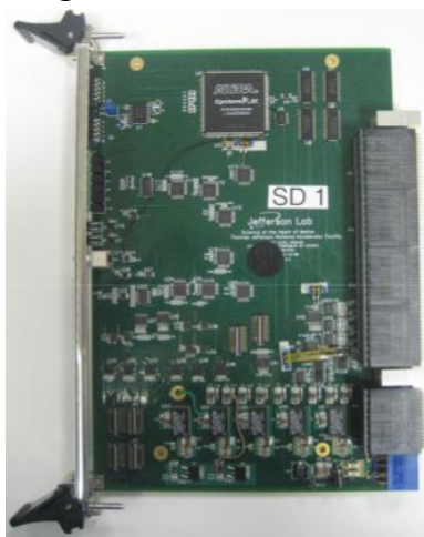
Signal Distribution Board
