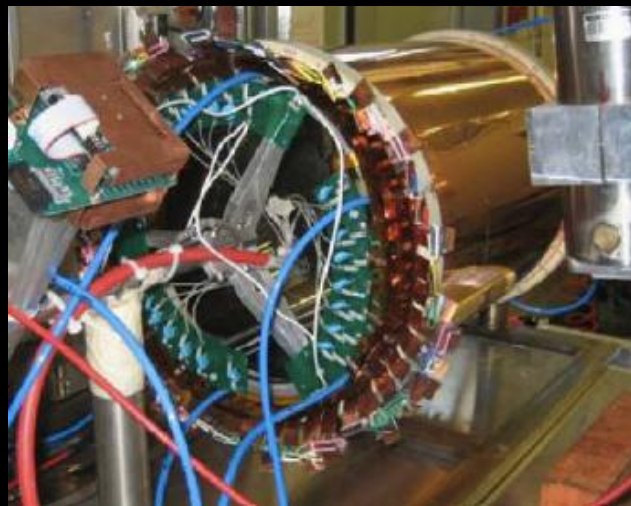
Cylindrical GEM Tracker for KLOE @ DAPHNE (Frascati, Italy)
