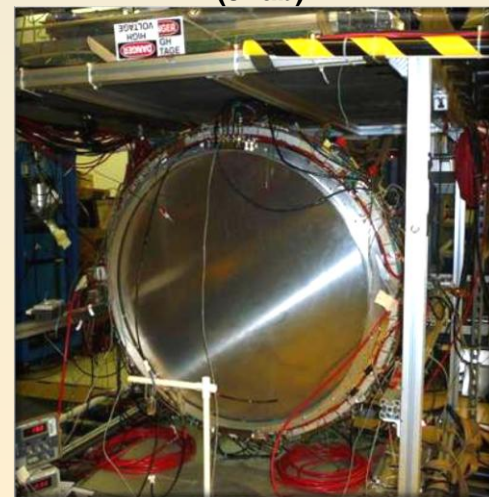
Forward Drift Chamber (JLab)
