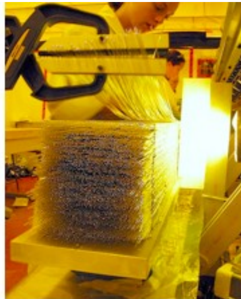
BCAL module being constructed
