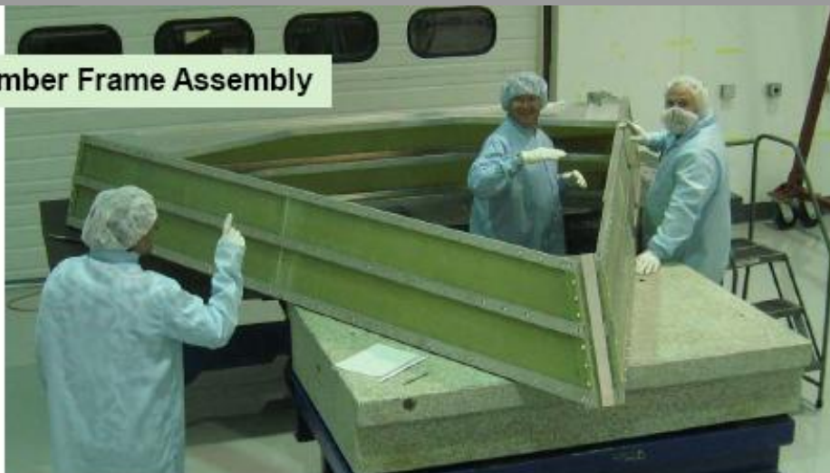
Hall C – Wire Stringing Jig for Drift Chamber
