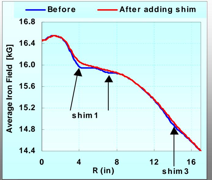
Iron shims were added to remove unwanted dips in the average iron field distribution at about 4", 7" and 14" radii
