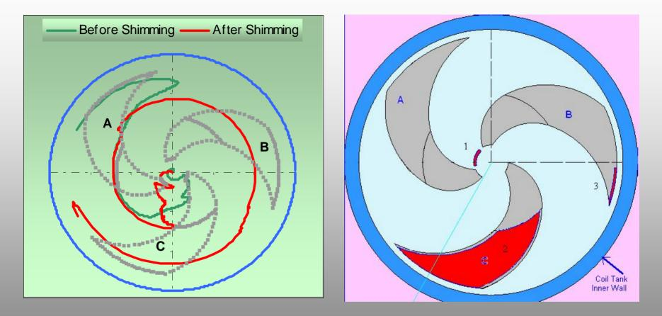
The positions of iron shims to be added are determined by the phase distribution of first harmonic component of the field.
