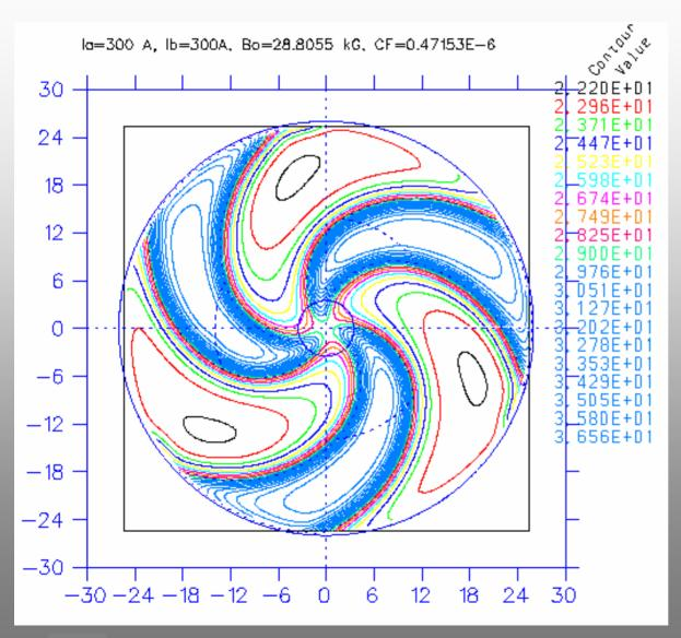
Three-fold symmetry dominated magnetic field distribution is characteristic feature of the three-sector geometry of the VECC K500 superconducting cyclotron
