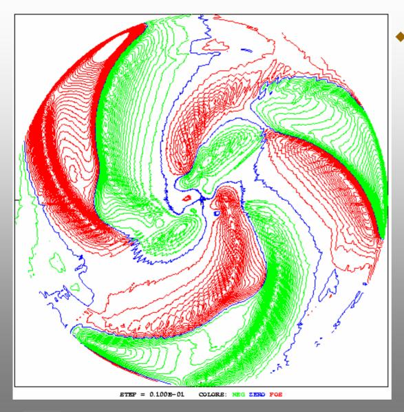
Deviation from perfectly three-fold symmetry arises out of manufacturing tolerances and assembly errors. The blue contour is of zero deviation, i.e. perfectly three fold symmetric data points, the red and green contours are of positive and negative deviations respectively with 10 gauss steps. This includes all harmonics other than 3rd harmonic and integral multiple of 3.(at l\_alpha= l\_beta = 300 Amperes)
