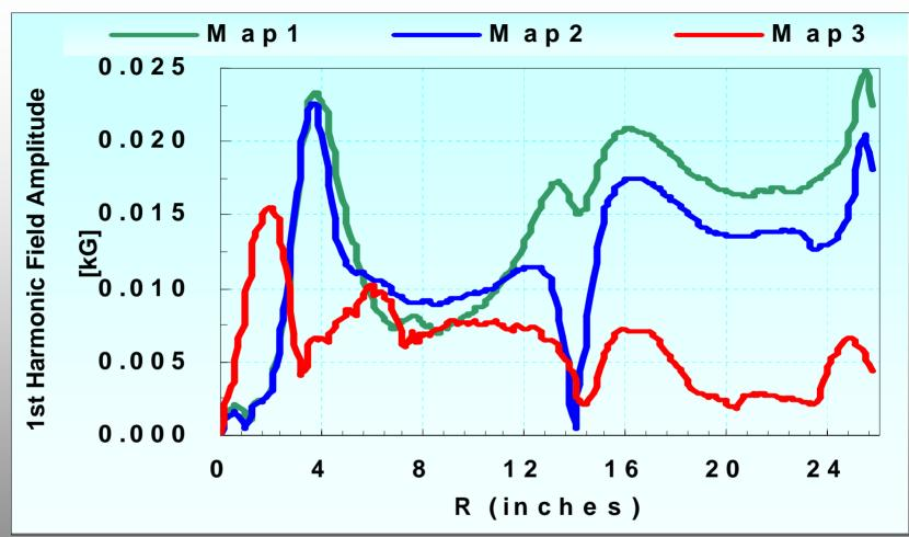
The aim was to reduce the error harmonics to manageable proportions at the important places by adding iron shims, however, to minimize the 1st harmonics at the extraction region was the most important issue.
