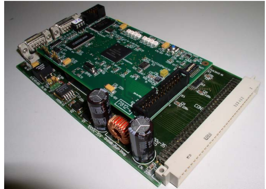
Coldfire-based controller board with CANopen-to-SEDAC adapter
