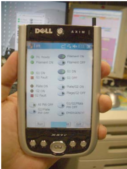
Figure 7: A prototype VI ported to PDA. This is the control panel for an RF power amplifier.
