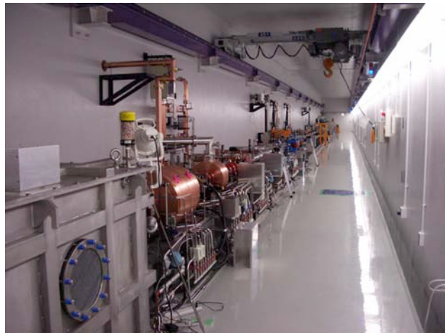
Figure 1: Cover shot of the SCSS prototype accelerator. From this side, 500kV Gun tank, 238MHz pre-buncher, 476MHz booster cavity are shown.
