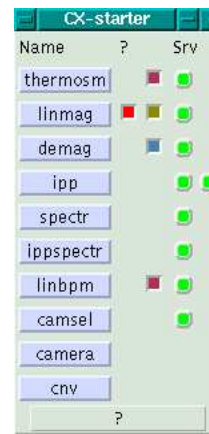
Figure 4: CX “control center” — CX-starter. Round leds in “Srv” column show status of appropriate device servers, square leds in “?” column signal channels’ status (cumulative for a subsystem).
