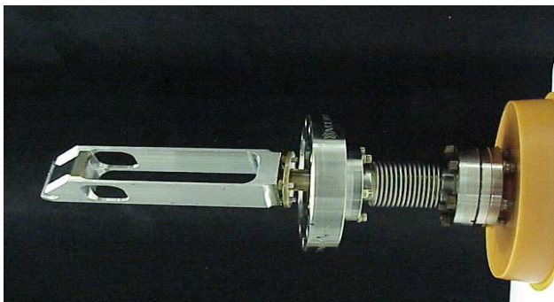
Figure 2. Adjustable mount of the SLI “in-vacuum” mirror.
