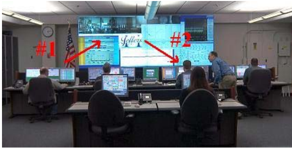
Fig. 3: Renovated MCC control room featuring the Display Wall. Operator #1 can “wall” an entry; later Operator #2 can “fetch” the entry, modify it, “re-wall” it or submit the entry to the logbook
