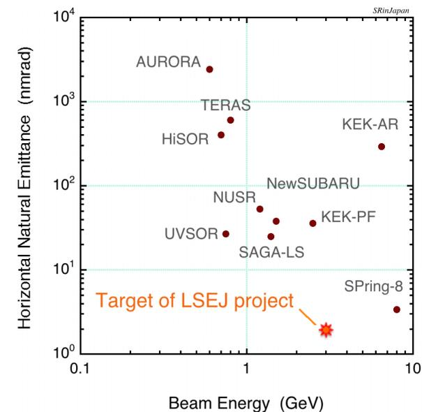
**An advanced low emittance 3 GeV machine for X-ray should be established in East Japan.**
