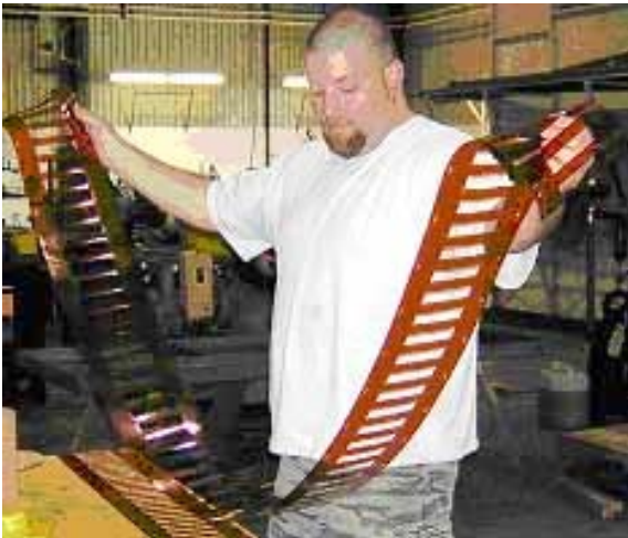
G. Biallas et al. an 8 cm period electromagnetic wiggler magnet with coils made from sheet copper", Proceedings of PAC 2005, Knoxville, 4093 ; FEL04, 554-557
