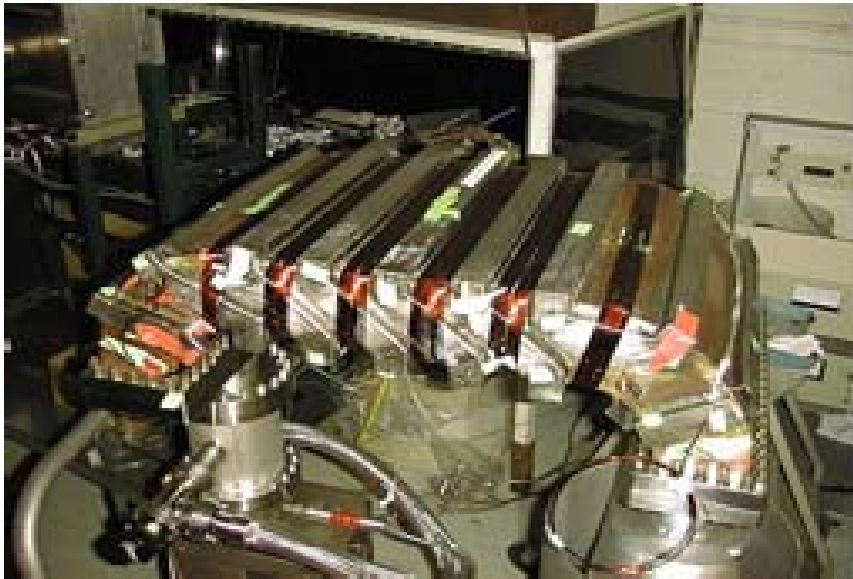
Solenoid coils on a reduce height waveguide to suppress multipacting (field ~30 Gauss)
