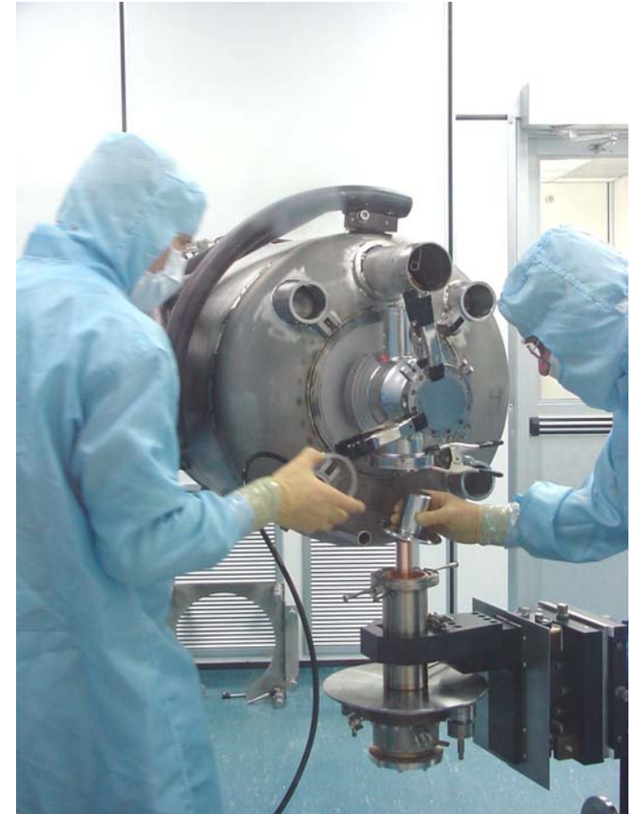
FPC assemble on a cavity
