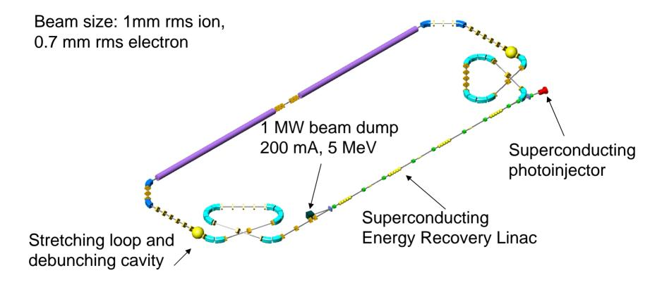
54 MeV electron beam for cooling 100 GeV/A (gold ions and protons. Must use superconducting Energy Recovery Linac. Need 20 nC electron bunches at 9.4 MHz. The emittance is challenging.
