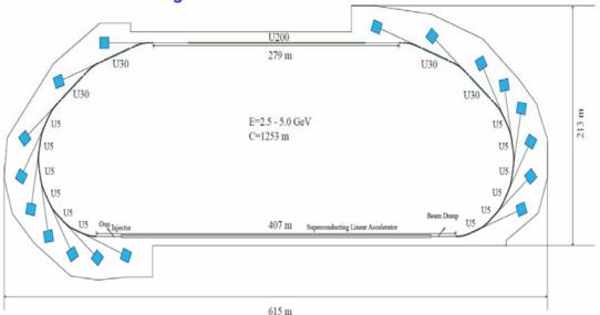
The dimensions of the 5-GeV KEK-ERL must be inside the KEKB rings at Tsukuba campus.
