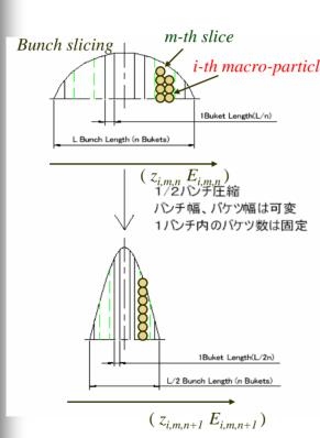
th slice The longitudinal motion of each macro-particle is developed i-th macro-particle in time evolution of a small time step ( $\Delta t$ ) using the energy and z-position relations of the i-th macro-particle within the m-th sliced bunch after the n-th small time step,
