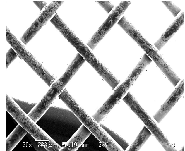
fig.3, H-terminated and B doped RF plasma preparation. Bright because of NEA Layer.
