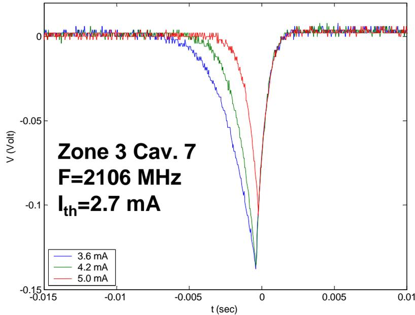
HOM power, measured by Schottky diodes, vs. time for  $I_b=3.6, 4.2,$  and 5 mA. The rise time depends on the beam current as
