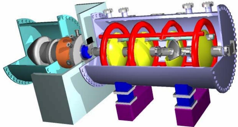
**JLab concept of a high voltage DC gun married to a low frequency rf cavity (shown here with SNS cavities)**
