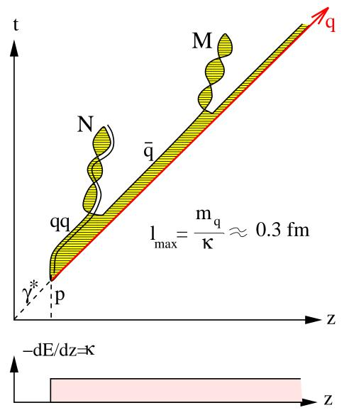
String tension provides a constant rate of energy loss
