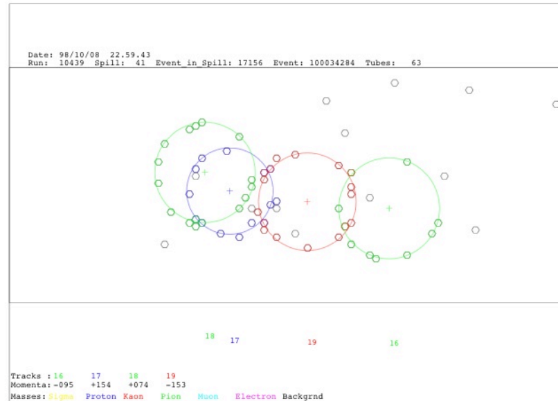
FIGURE 14. Single event display. The small hexagons represent a hit phototube, the circle shows the ring for the most probable hypothesis, and the numbers denote the track numbers, with their momenta shown at the bottom.
